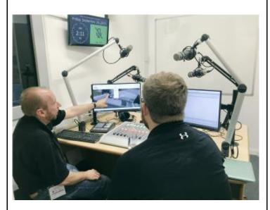
Based upon a standard package and with a few adaptations to the particular needs of the University, the integration of the automation system and the AEQ CAPTIOL IP console is seamless since the control protocol for the CAPITOL IP for, for example Fader status, Vu-meters, Fader starts/stop and Virtual GPI/O's, are embedded into the SW solution from Broadcast Radio.
