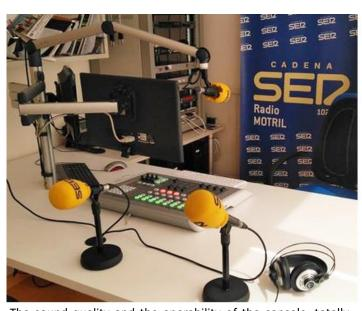
The sound quality and the operability of the console, totally adapted to local stations, allows the same mixer to work simultaneously with several ONAIR programs while preparing the local disconnections or contributions. These features made AEQ CAPITOL IP digital audio mixers the perfect solution for many radio stations that have multiple programs and need to optimize technical and economical resources.
