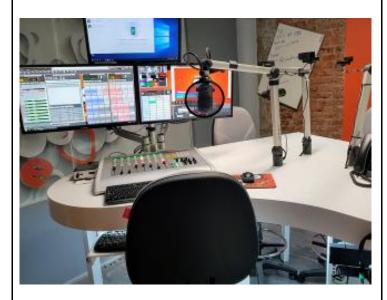
AEQ CAPITOL IP incorporates all the basic features that are usually required in broadcast applications: automatic monitor mute, cough-cut, fader-start, signaling control, control signals for the automation of external devices, external communications management, intercom, etc.
