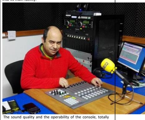
The sound quality and the operability of the console, totally adapted to local stations, allows the same mixer to work simultaneously with several ONAIR programs while preparing the local disconnections or contributions. These features
