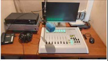
From there, editors can do remote interviews over telephone and other editing tasks. Also, given the full functionality of this high-end broadcast console, and its IP connectivity with 16 inputs and 16 outputs to the BDN main IP network, some small break bulletins can be broadcast from here now
