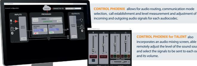
**CONTROL PHOENIX for TALENT also** incorporates an audio mixing screen, able to remotely adjust the level of the sound sources and select the signals to be sent to each output and its volume.
