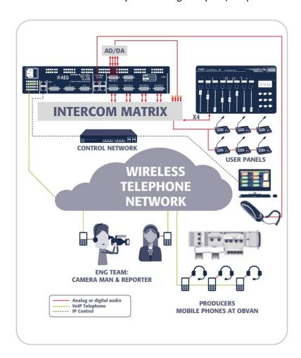
The operator establishes the communication with the remote parties using a handset. The intercom matrix establishes bidirectional routings with the console and complex party-line routings with different panels according to each production's requirements.
