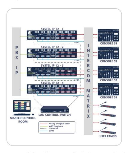
When the operator presses it, it provides a command to the Intercom matrix so it establishes a bi-directional route with the corresponding console or intercom panel using a pre-programmed circuit. When the call is hug, the GPO button is deactivated until a new call is established. The ON
