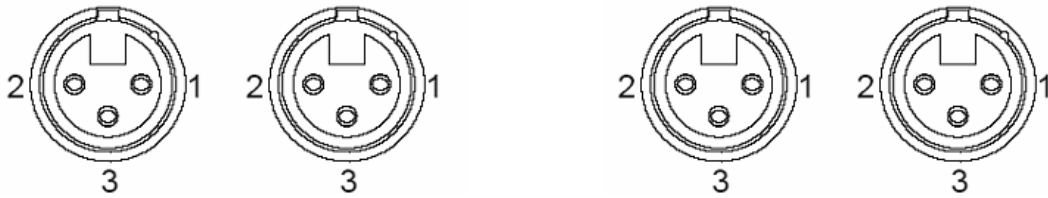
XLR 3p Female-panel Pinout
