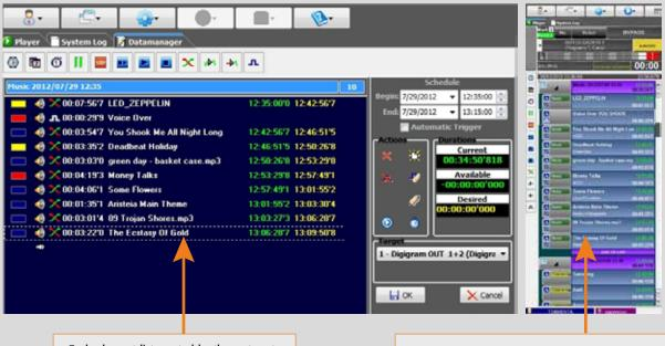
Each play-out list created by the system to cover a time window is shown to the operator together with its play-out schedule and the time allocated for each audio item so it can be revised and edited as required.
